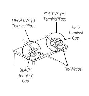
Detail "C" - Installing Battery Terminal Cap onto Battery Cable
